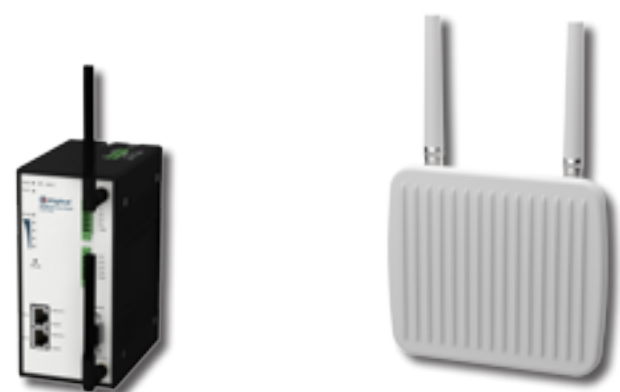
WLAN Access point IP30
